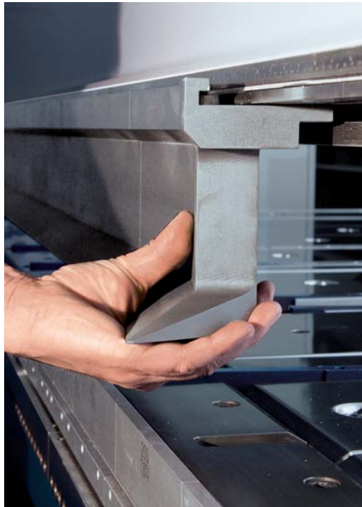
The hydraulic tool clamping device on the clamping beam reduces set-up times.
