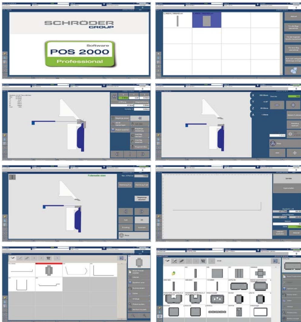
Graphic control POS 2000 Professional: The result is always in front of your eyes – from the first steps to simulation.
