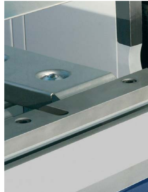
The lowerable folding beam is necessary to bend bigger radii with high precision. As an option, a motorized folding beam adjustment is available, controlled by the graphic control POS 2000 Professional.
