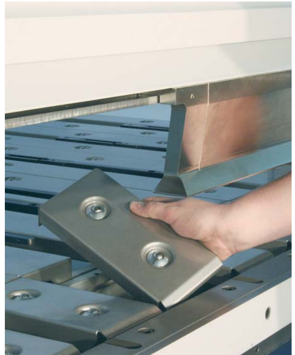
The removable pans make room for down-flange applications.
