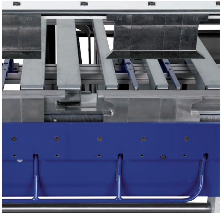
Ingenious patent: with the fast eccentric clamping device tool changes can be done with ease.
